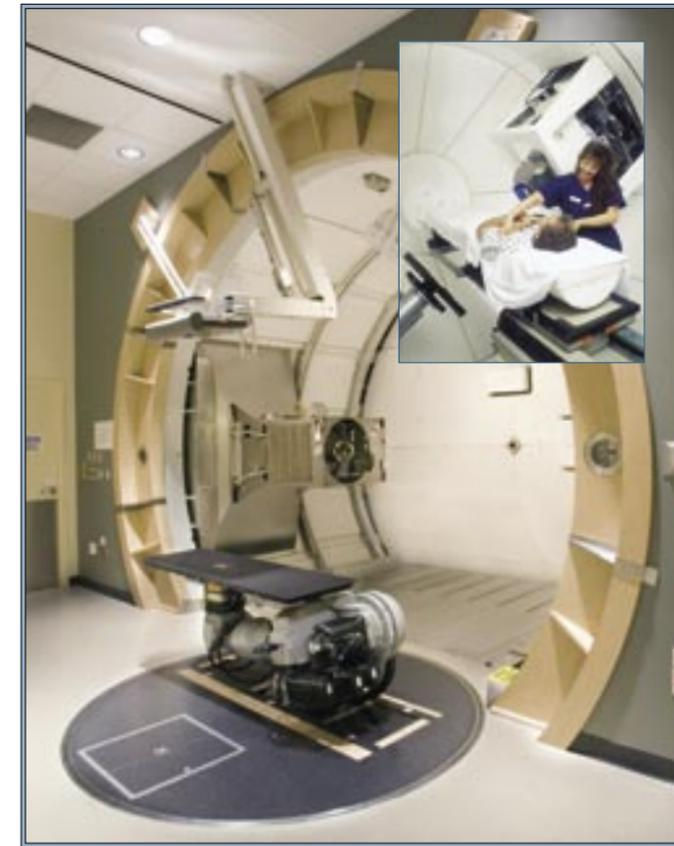
In 2007, the Midwest Proton Radiotherapy Institute (MPRI) treated the first patient in the world using an industrial robotic patient-positioning system with a rotating gantry, so protons aimed at the tumor can enter the patient's body from multiple directions. Since 1954, when proton therapy was first introduced for human treatment, about 55,000 patients have been treated in the U.S. and around the world.
